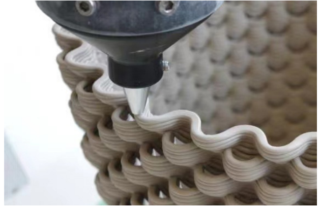
Figure 6. 3D printing molding
