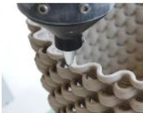
Fig.6 3D printing molding
