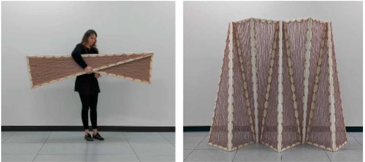
Figure 3. Final wall being transported and deployed. ↩
