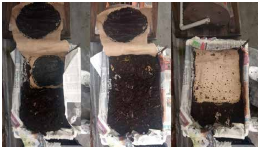
Figure 2. Step-by-step photographs showing how to place boihis̄sa-ata 's material draft into a box of compost soil for testing. Steps from left to right: (1) a hole is dug and the anode is placed inside, (2) the anode is covered with soil, (3) the cathode is placed over it.
