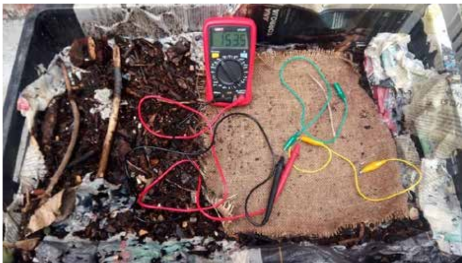
Figure 3. Measuring the electrical power released by the bacteria living on βoihissa-ata's material draft. The multimeter measures 153.5 mV of a microbial fuel cell in an open cell configuration. An open cell configuration means there is no resistive load connecting the anode and cathode.
