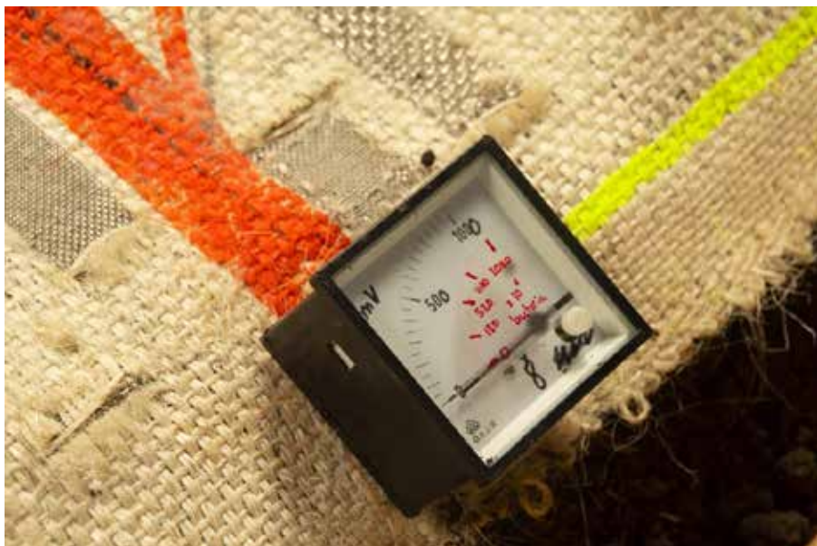
Figure 5. A photograph of boihis̄sa-ata 's voltmeter which has been adapted to translate the electrical power of the bacteria to display an estimate of their population.
