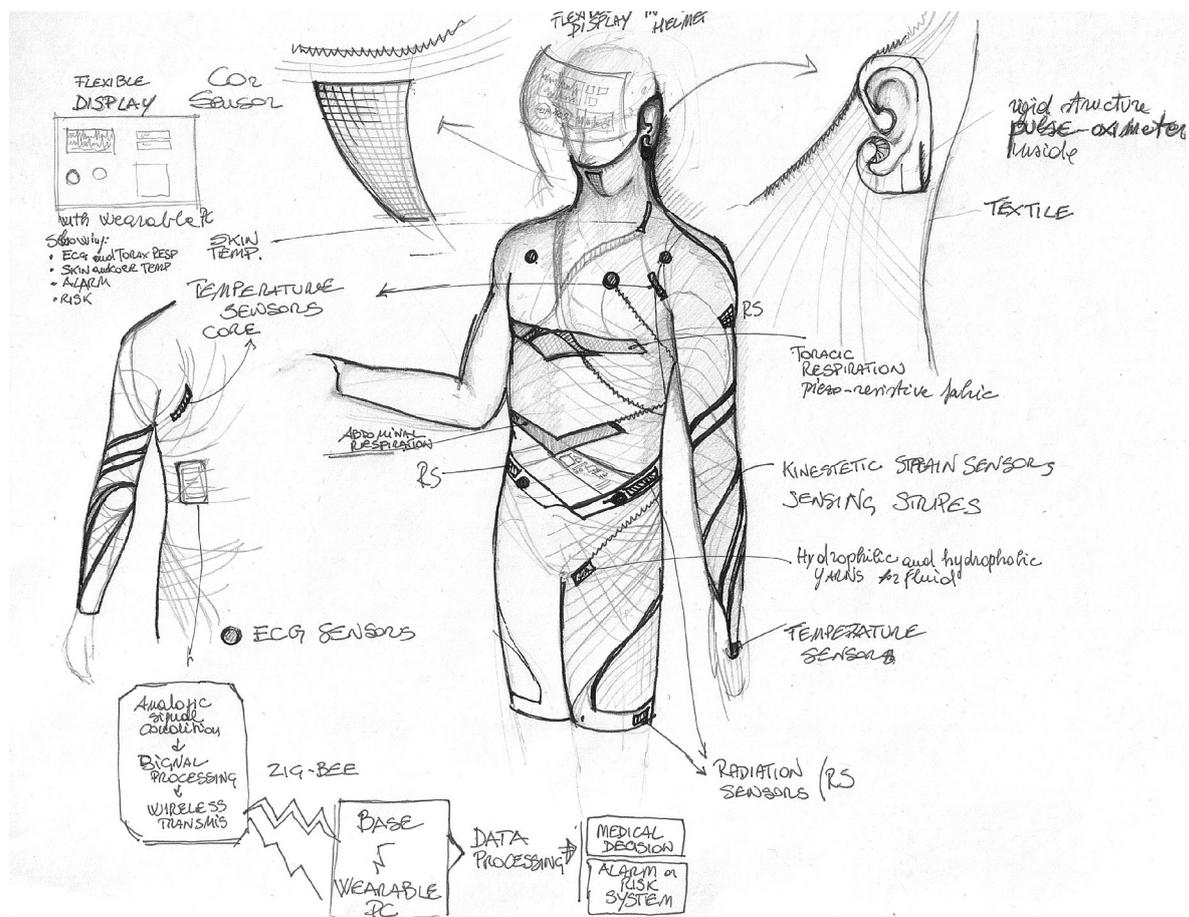
Figure 1. Concept of the wearable systems
