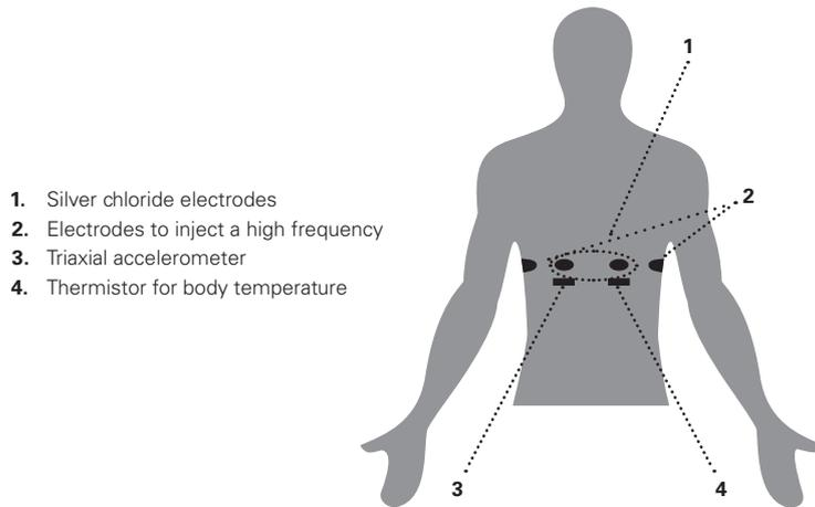
Figure 2. Scheme of device
